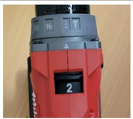
Put cutting oil over the location and put the drill on the screwdriver setting.
